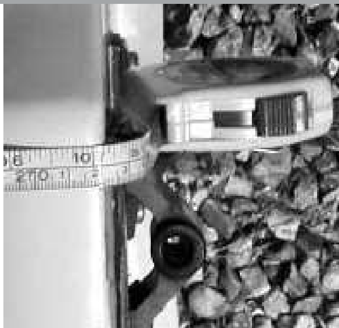
The position where measurements are taken to (back of hull at transom/gudgeon). In this case the measurement from base of mast = 272 cm.
